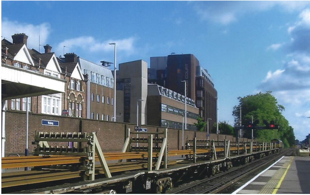
Figure 21.2 One type of special Freight train is an Engineering train, which is a train for the conveyance of materials or equipment to locations where railway maintenance work is to be carried out. The train in Figure 21.2 is conveying long rails to a location where they will be welded together to form Continuous Welded Rails (CWR) See Section 14.
