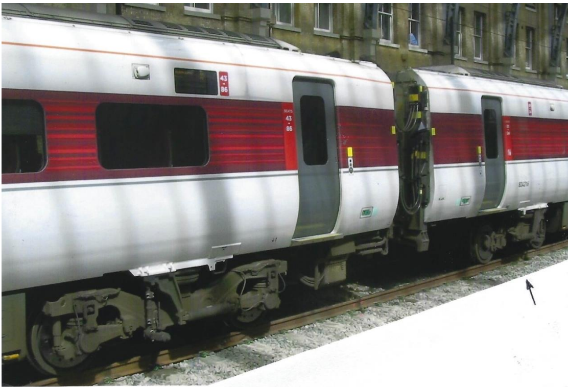
Figure 17.9 The steam engine's power is in the 3 sets of large driving wheels (i.e. 6 wheels). The LNER AZUMA'S power is in certain coaches. For instance, in the above photograph, the bogies on the left hand coach are powered, whereas those on the right hand coach are not powered (trailer coach).
