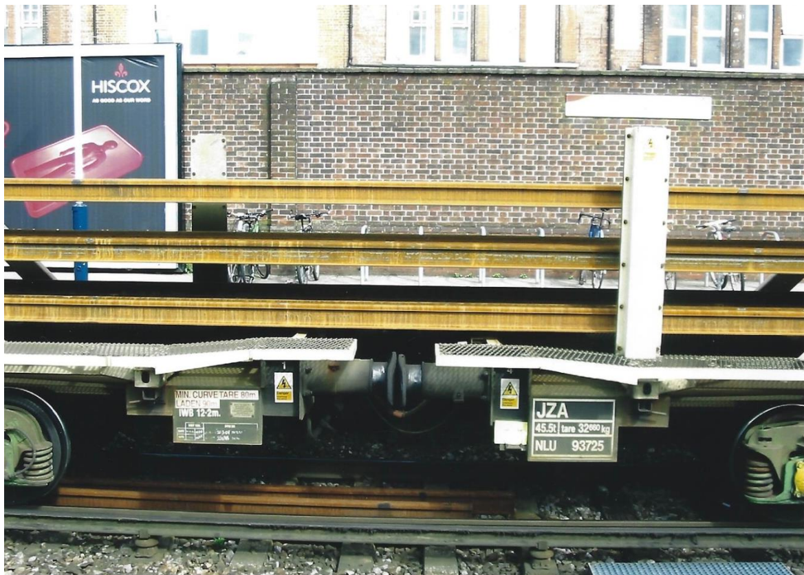
Figure 21.3 When the train is on curved track, the long rails bend with the train, which is another example of steel's ability to be flexible within limits. (See Figure 15.1 )
